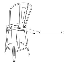
2>Pull down the back.Make a obtuse angle between the back and the seat and then assemble the rest two screws on the seat.
