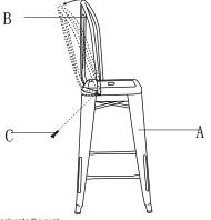
1> Fasten the back onto the seat.
